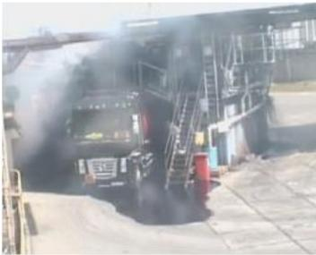
Still from CCTV footage of an eruption of bitumen from a tanker.
